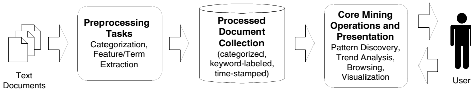
Figure I.4. High-level text mining functional architecture.
